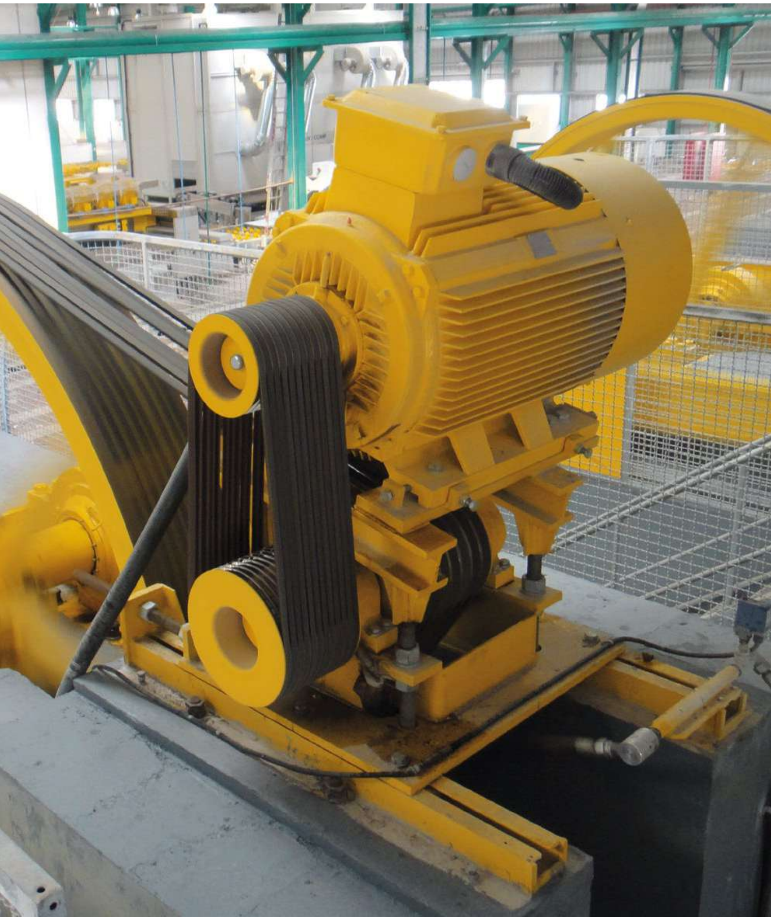
Above: detail of the double connecting rod system and multiple belt transmission as to guarantee the best levels of tensioning and traction.
