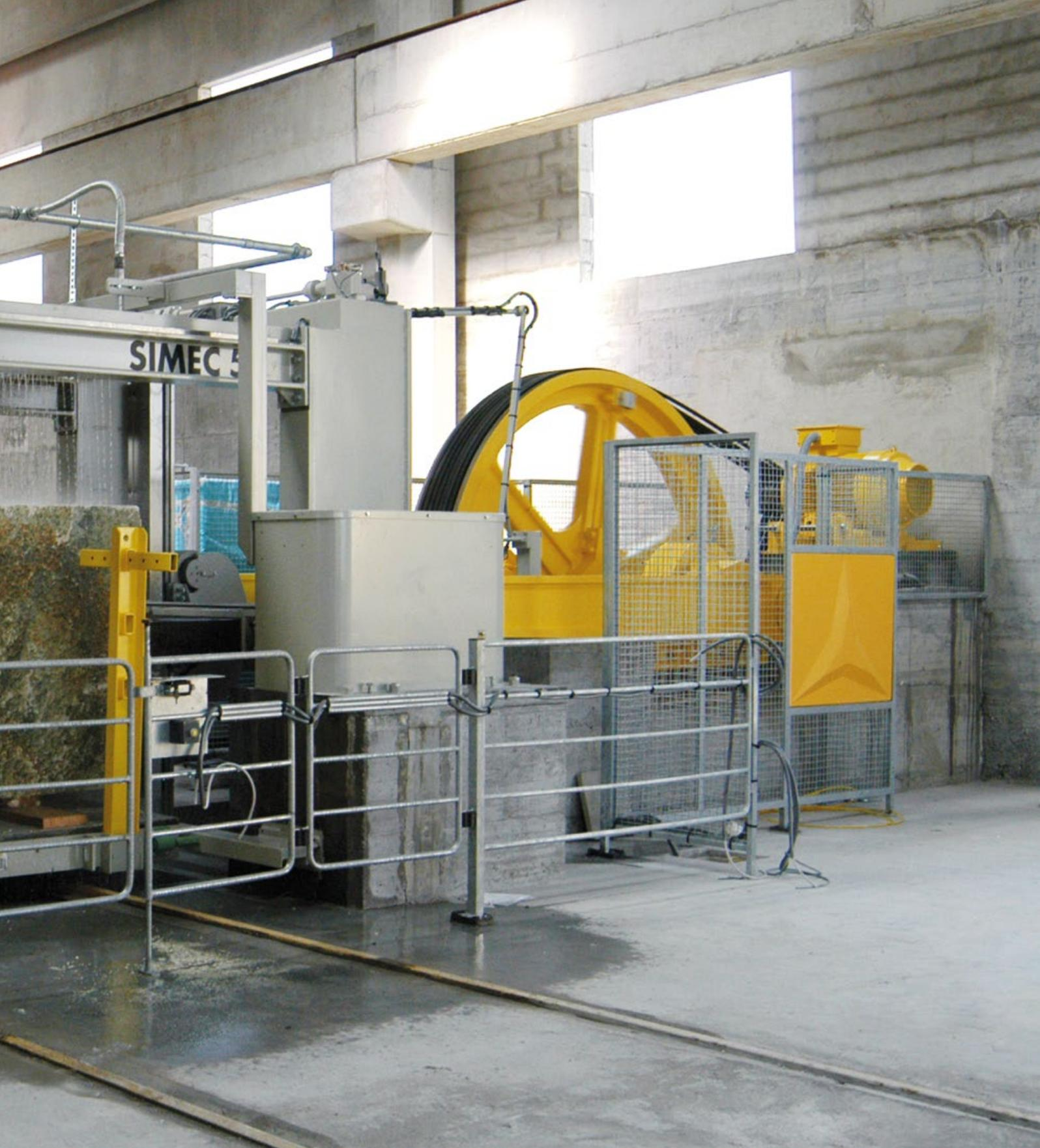
Sopra: telaio M50 - Above: M50 gang saw
